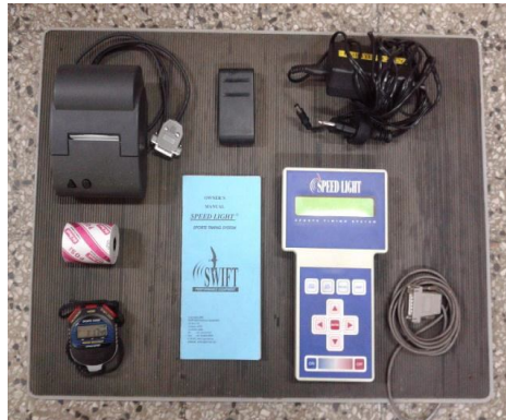
Figure 1. Portable Contact Timing Mat System (Thermal Printer, Thermal Paper, Stop Watch, Contact Mat, Data Cable, Data Recording Unit)
